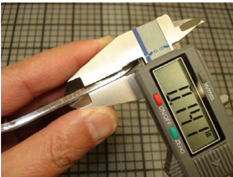
The width of the fold measures at .141 inches. Multiply this number times the length of the cover plate at 2.81 inches, and then double that for two plates. Your conclusion should match mine. Over 3/4" of metal will block your sound.
